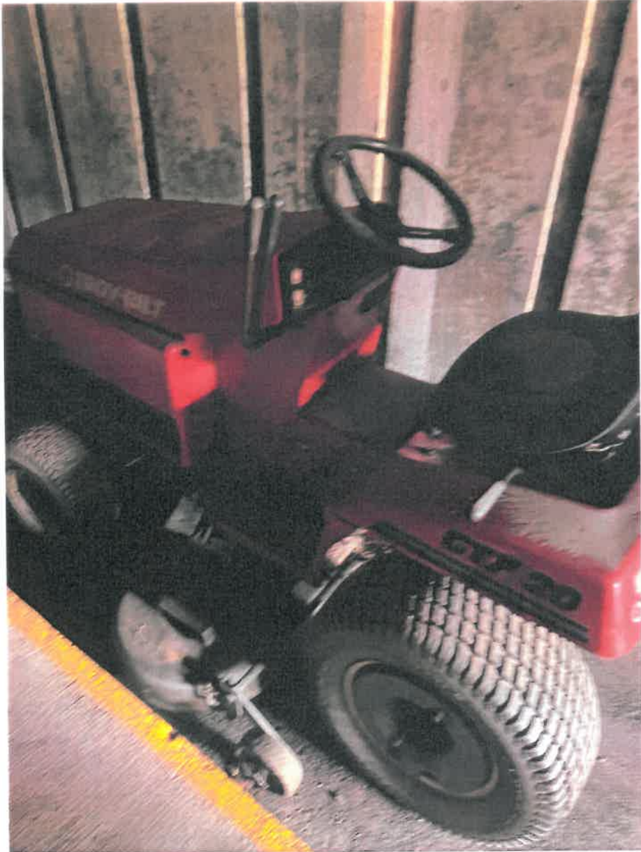
22- Lawn Tractor Stored in UV Building (Snow blowing Equipment in Front of Lawn Tractor Out of View) Note Silt on Top of Engine Cover From Being Completely Submerged
