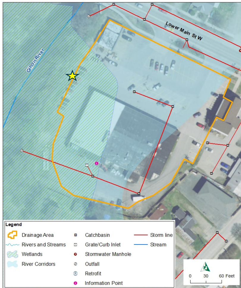
Figure 12. The drainage area for the proposed BMP is shown in orange. The proposed BMP location is shown with a star.
